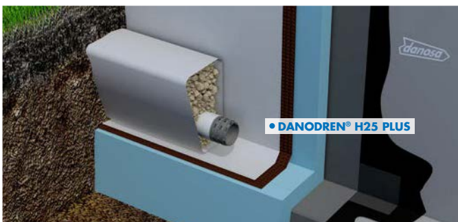
Flexible walls with (SBS) waterproofing.
